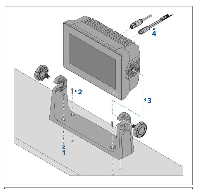
**Note:** The illustration depicts an Axiom<sup>™</sup> 7 being mounted on a plastic trunnion bracket. The trunnion bracket supplied with the Axiom<sup>™</sup> 9 and Axiom<sup>™</sup> 12 are made from metal and so look different than the trunnion shown. A metal trunnion bracket is also available for the Axiom<sup>™</sup> 7 as an accessory; Part number: R70524.
